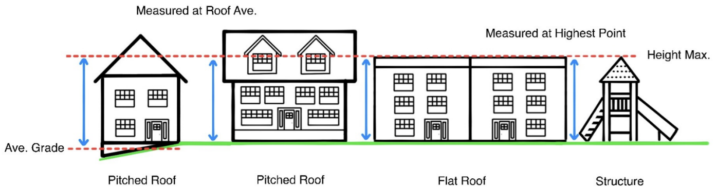
Figure 3-1 Building and Structure Measurements
